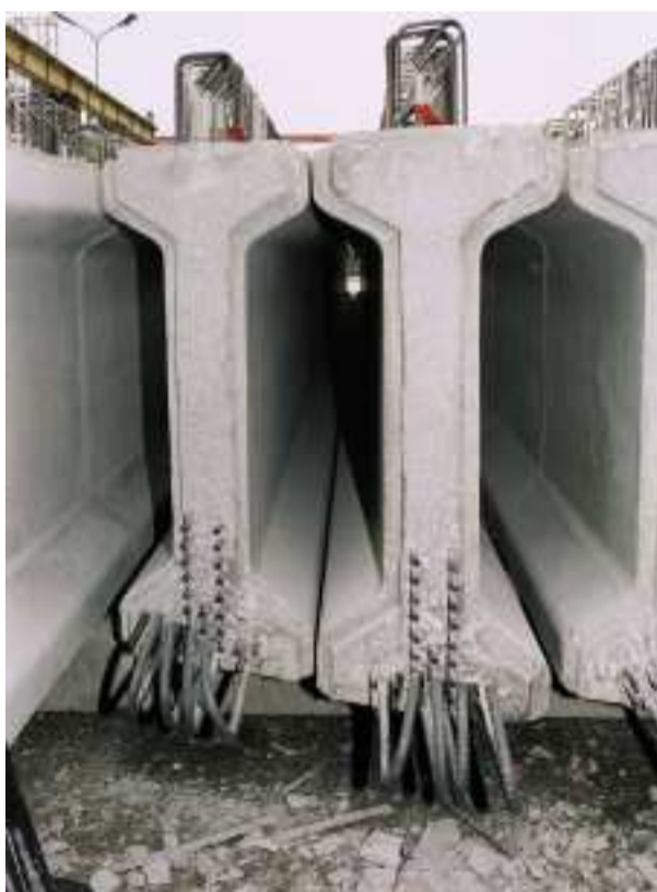
L'INDUSTRIELLE DU BÉTON specialises in the prefabrication of long beams.
